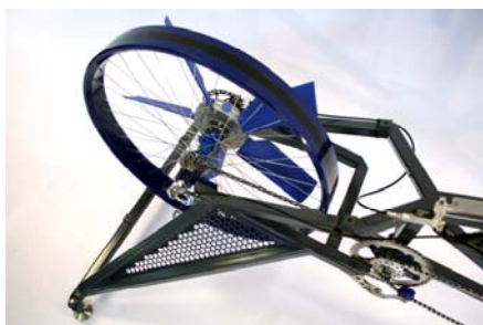
Fly Wheel fan Assembly to simulate inertia and drag
